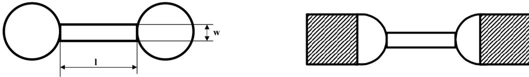
Cross-hatched surface is of high-conductive varnish and  $\rho^{lak} = 10^{-4}\rho$ , semicircular segment and bridge are of conductive paper and  $\rho$  resistivity. Semicircular segment is of  $D$  diameter.
